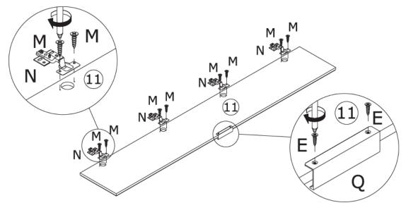
Fix handle(Q) with screw(E) as shown.
