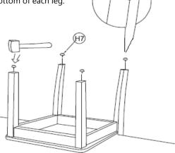
a) Assembly from STEP 1, bottom-side up as shown on an elevated surface (e.g. table top).
