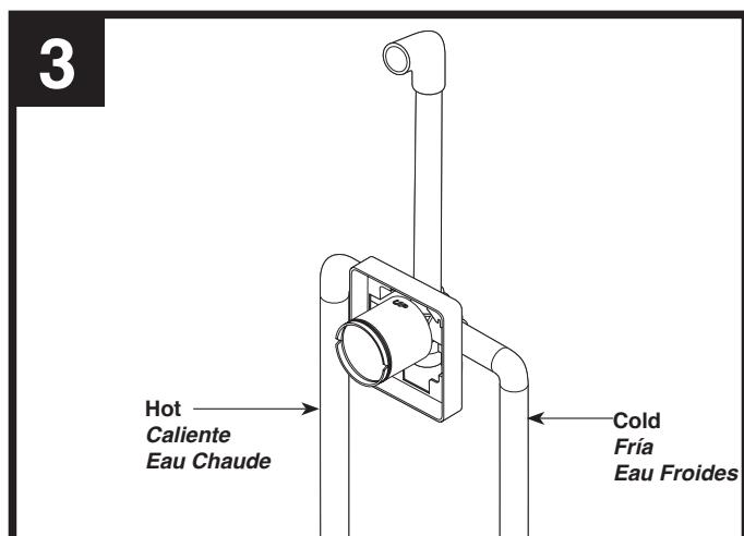
Connect water supplies to left (hot) and right (cold) valve body inlets. Iron pipe connections are shown; however, copper pipe may be used with proper adapters.
