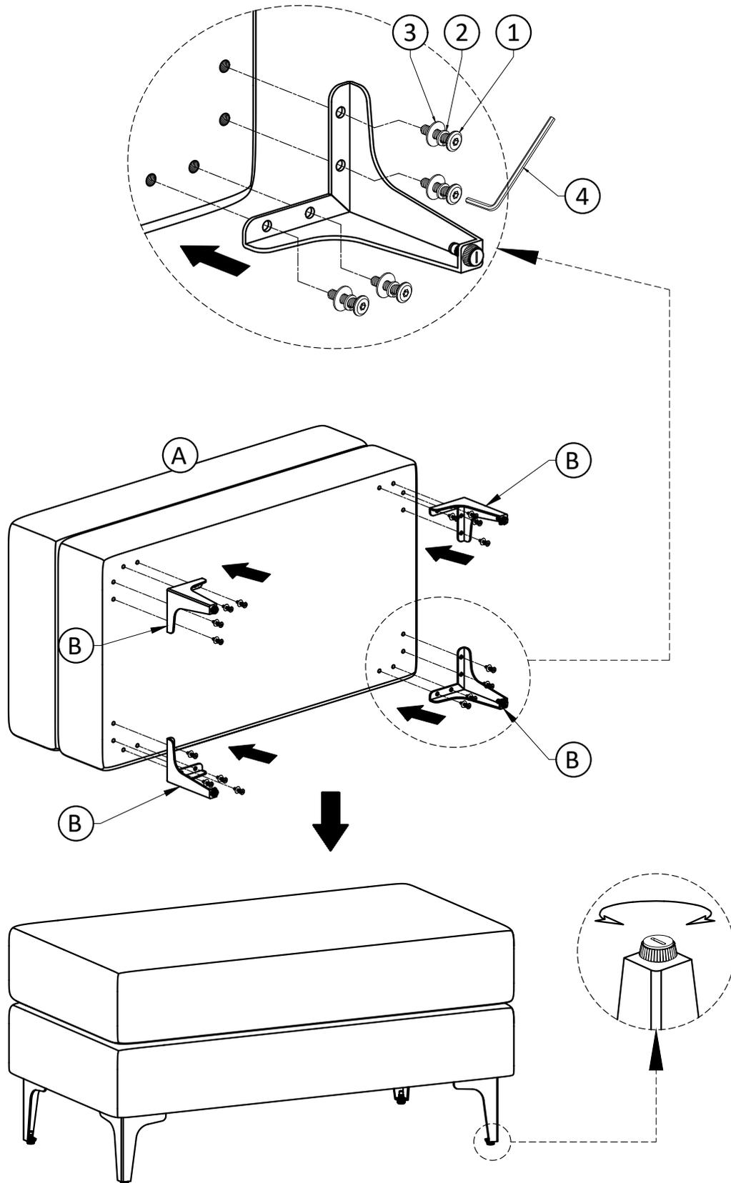
1. Attach Legs (B) to Ottoman Seat (A) using Bolts (1), Lock Washers (2) and Washers (3) through guide holes.
