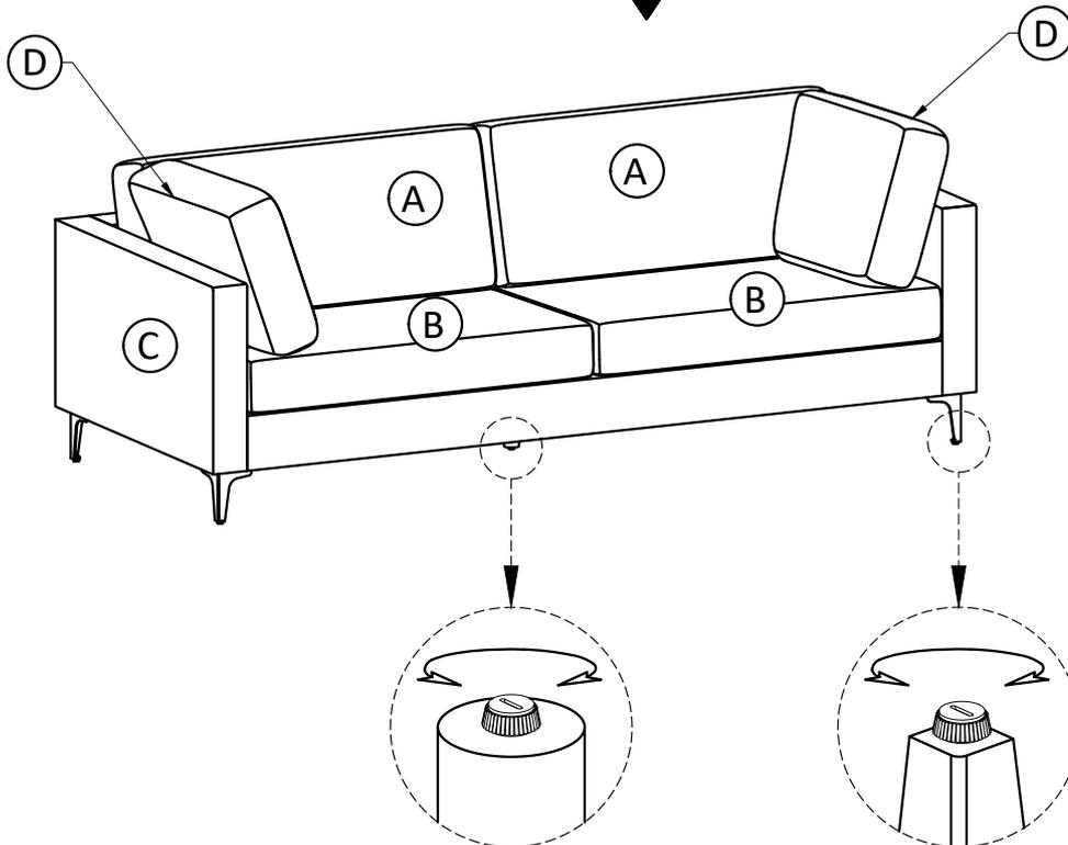
Note: Levelers on bottom of legs can be adjusted if floor is uneven.
