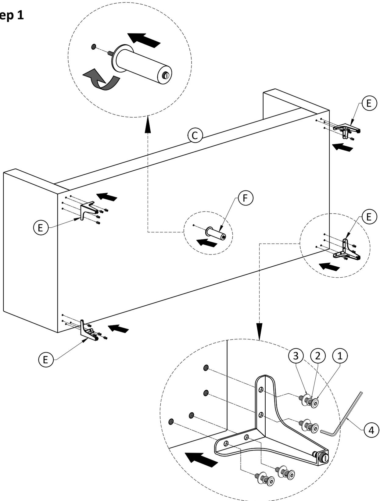
1. Attach Legs (E) to Sofa Seat (C) using Bolts (1), Lock Washers (2) and Washers (3) through guide holes.
