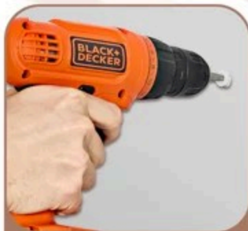
Drill Anchor into Wall
