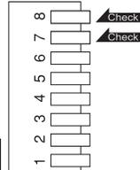
The power must be unplugged when adjusting the dip switches to switch the airflow amount.
