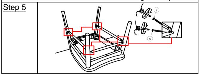
Attach Stretchers to Back Rest(A), Front Leg(C) and Front Leg(D) using Screws(6) with Screwdriver(8). Then, Attach Front Rail to Front Leg(C) and Front Leg(D) using Screws(6) with Screwdriver(8)
