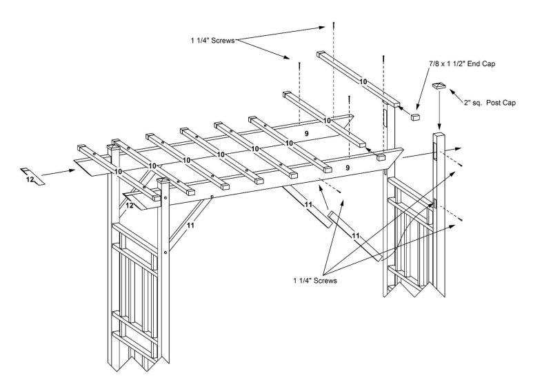
Insert two 18" corner braces (part 11) into each 72" arbor top (part 9). Slide ends of arbor top rail through holes at top of post, inserting corner braces into posts. Measure 9 inches from tips of arbor top rails and slide posts so outside of post in 9 inches from end of arbor top rails. Using three 1¼" screws per post, fasten together posts, arbor top rails and corner braces.
