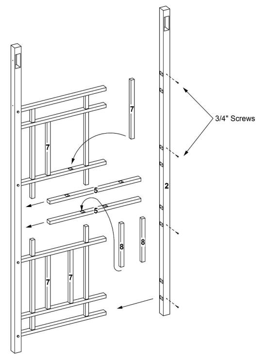
Insert two 27½" middle cross rails (part 5) into remaining routed holes in side of post, inserting free ends of 26½" vertical rails into middle cross rail. Insert four 16¾" vertical rails (part 7) into remaining holes in inside cross rails. Insert two 13" vertical rails (part 8) into remaining holes in middle cross rails. Insert free ends of cross rails into one 84" right post (part 2).
