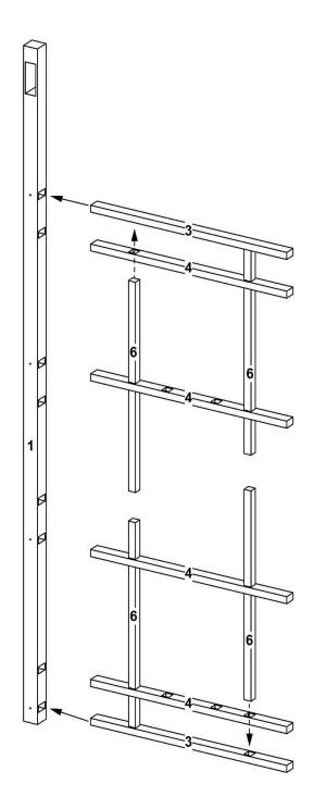
Starting at bottom of one 84" left post (part 1), insert one 27½" outer cross rail (part 3) and two 27½" inner cross rails (part 4). When inserting two inner cross rails insert sides with four routed holes facing each other. Insert two 26½" vertical rails (part 6) through outer holes of inner cross rails and into outer holes of outer cross rail.
