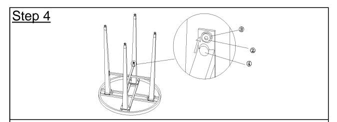
Now fully tighten all Bolts at all joints in a sequential manner.
