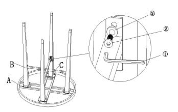
Attach Connector(C) between Legs(B) using Bolts(2) and Washers(3) with Allen Key(1) as pictured.
