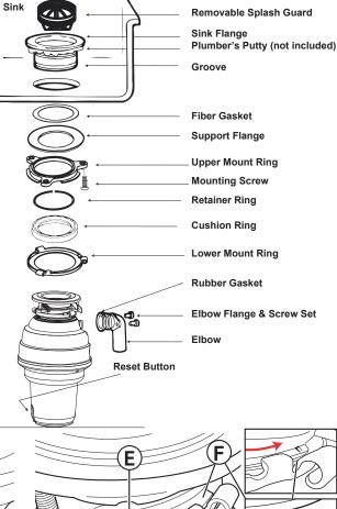
As the Lower Mount Ring is turned counter clockwise each tab slides up onto the Upper Mount Ring Ramp (E) and locks in position over the Ridges (F).
