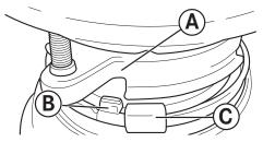
The lower mounting ring (which is part of the disposer) has 3 tabs that grab the mounting ring ramp.
