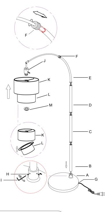
PARTS DIAGRAM: (1) Hex Wrench 1. Locate the small allen wrench (  $\rm I$  ) and set this part aside for use later in these instructions.
