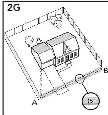
**Sample 4 (2G): Front Boundary Only (Double Loop)** From the Fence Transmitter, run the wire to **A**, **A** to **B**, **B** back to **A** keeping the wire separated **at least 5 feet**. Twist the wire from **A** back to the Fence Transmitter.
