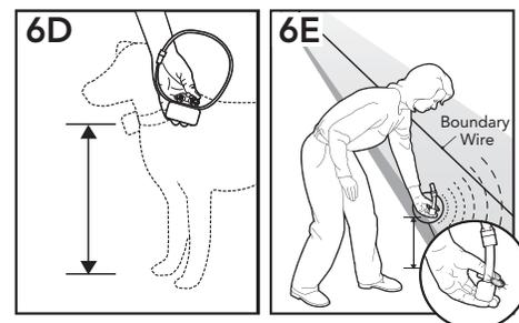
7. Test in a number of different locations around the containment area until you are satisfied that the system is functioning properly.
