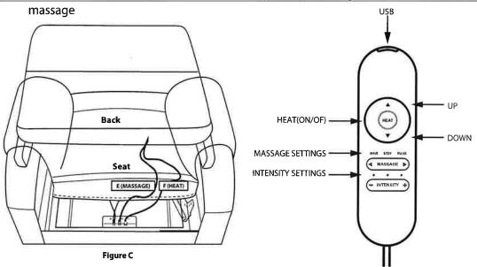
Press the MASSAGE  $\prec$  or  $\blacktriangleright$  button to go to the three available massage setting: WAVE, STEADY, or PULSE. Each setting is indicated by a COLORED LED light. The massage function will automatically shut off after 30 minutes of continuous use.
