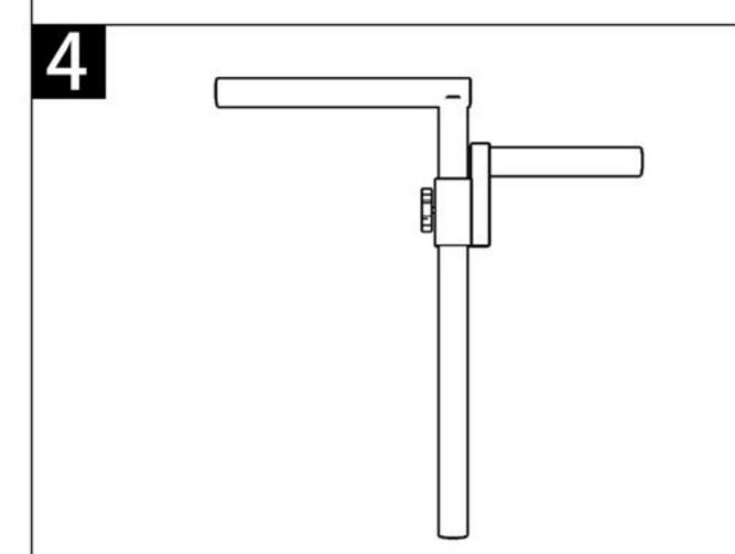
1.Put the pipe-shaped bracket on the 7-shaped steel pipe and fix it with the adjustment button
