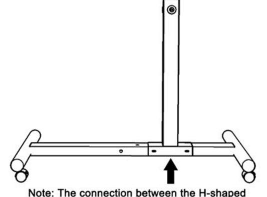
Note: The connection between the H-shaped steel pipe and the support rod must be screwed into a 6\*35 flat head screw from the bottom (pointed by the arrow).
