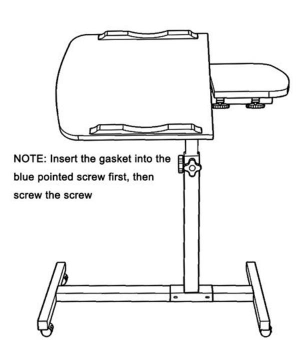
Install the desktop baffle: Secure with blue pointed screws and spacers
