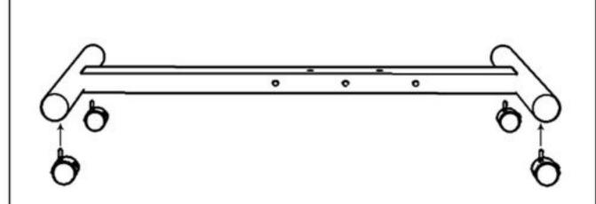
Install the wheels: Install the wheel to the H-shaped round steel pipe with a wrench
