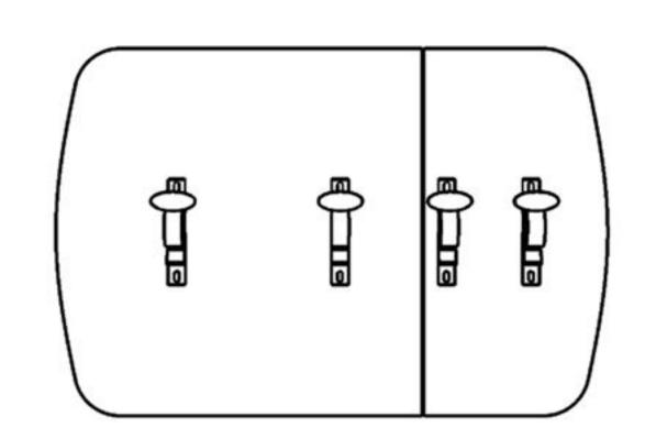
Install the Q-shaped bracket: fix it with 6\*12 flat head screws (the shortest flat head screw)
