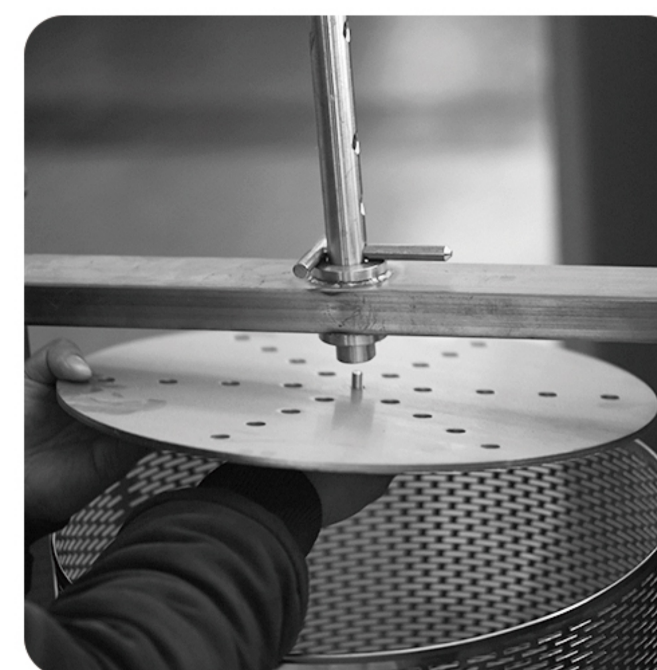
④ Take the screws to install the pressure plate on the pressure rod
