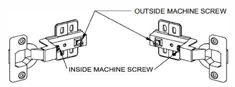
In the event that the door does not align properly, the INSIDE Machine Screws located on the Hinges are for adjusting slightly to the Left or Right. **DO NOT LOOSEN THE OUTSIDE MACHINE SCREW FOR ADJUSTMENT.**
