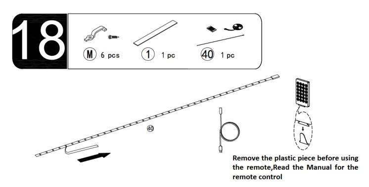
Please tear off the adhesive paper behind the light strip before pasting the light strip to part #5
