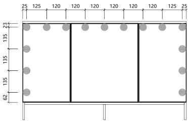
Mark the position of the bulb on the mirror plate according to the size in the picture. Stick bulb to correspoding positions on mirror plate.
