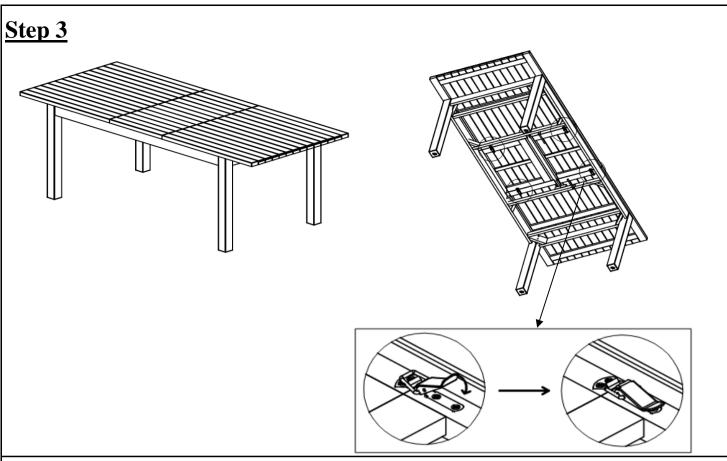
Lock the Metal Fastener under the table to lock the Expansion Board of Table Top (B) into place.
