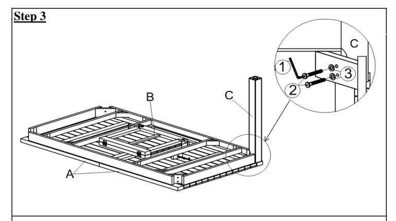
Attach one of Legs (C) to Table Top (A) by using 2 Bolts (2), 2 Washers (3) and Allen Key (1).
