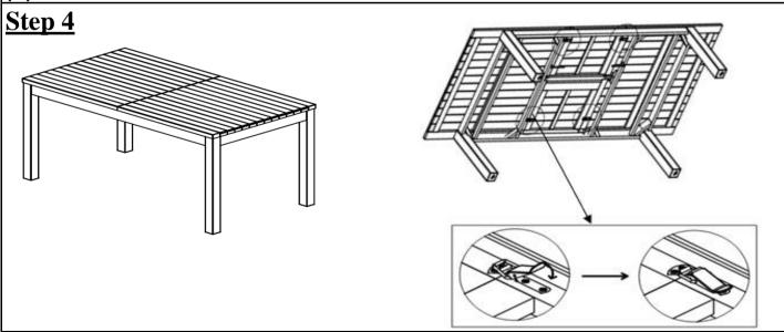
Lock the Metal Fastener under the table to lock the Expansion Board of Table Top (B) into place.
