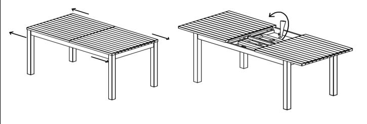
Gently pull the Table Top (A) outwards to open and stop when it could see the extension board frame support.
