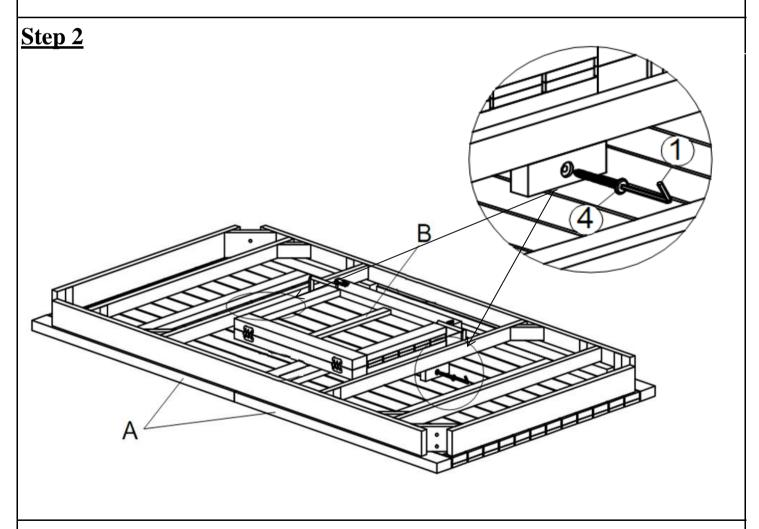
Put the Expansion Board of Table Top (B) into the Table Top (A) Then, secure Expansion Board of Table Top (B) with Table Top (A) by using 2 Screws (4)+ Allen Key (1) as designated points as picture above.
