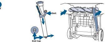
Replace the brush roll and belt by looping the belt over the motor shaft and the brush roll. Line up the end caps and pull the brush forward into place. This will stretch the belt. Return bottom cover back on and replace the screws.
