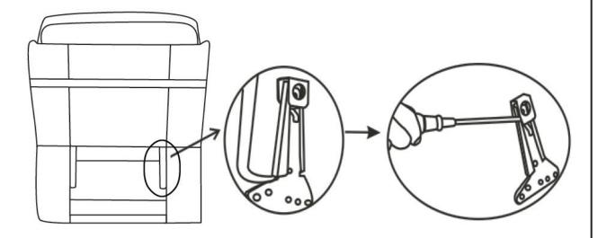
Please find a strong tool to prod the small piece of meal grooves, then the backrest will be pulled out. The tool is not included.
