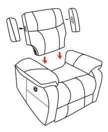
Insert the back ear (C) into the backrest (B):
