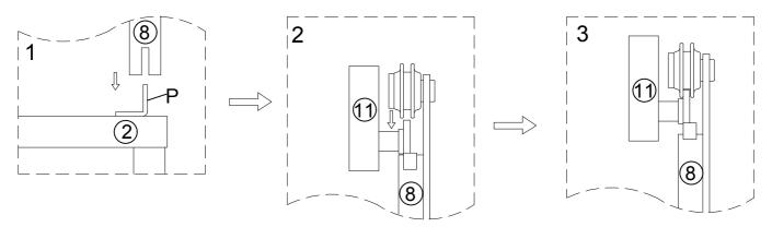
Part 2--Bottom frame Part 11--Door track Part 8-Sliding door Part P--Angle bracket
