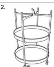
Expand the base into position after the middle and bottom trays are placed.
