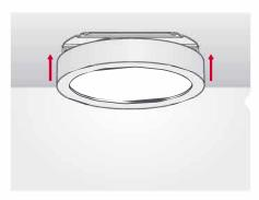
STEP 5: Push and feed all wires up into junction box as you raise the fixture into place.
