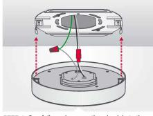
STEP 4: Carefully push connections back in to the J-Box, Align the two clips and driver on the fixture body to the opening of the J-Box Mounting bracket.
