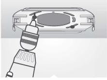
STEP 2: Attach the bracket to junction box using 2 screws (provided). Pull the AC cable with connector trough the bracket center hole.
