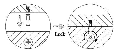
Use a flat blade screwdriver to tighten the cam nuts. A quarter turn clockwise is all that is needed.
