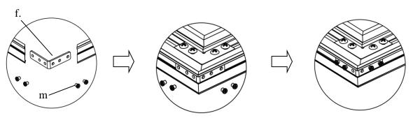
Step 12: Install the *angle cover* (n) on each corner of the frame using the M4x4 screws (m).
