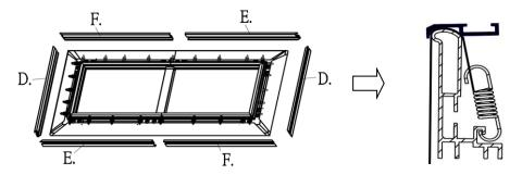
Connect edge trim frames (e/f) together using the M4 center joint (e) and secure with four of the M4x4 screws (m) as show in Step 1. Repeat for other side.
