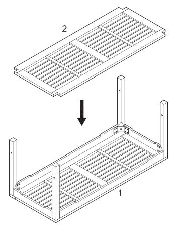
Carefully slide shelf (2) into place. (Shelf (2) will align with the pre-drilled holes of the table legs.)
