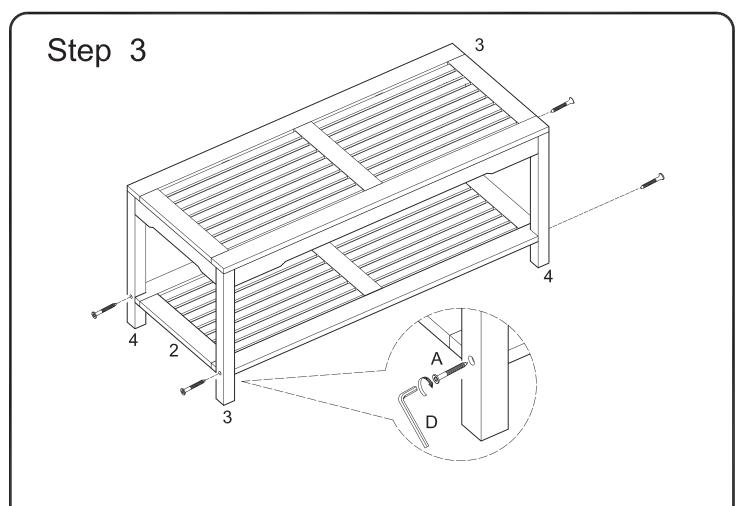
Secure shelf (2) to legs (3,4) using screws (A). Tighten screws (A) with wrench (D).
