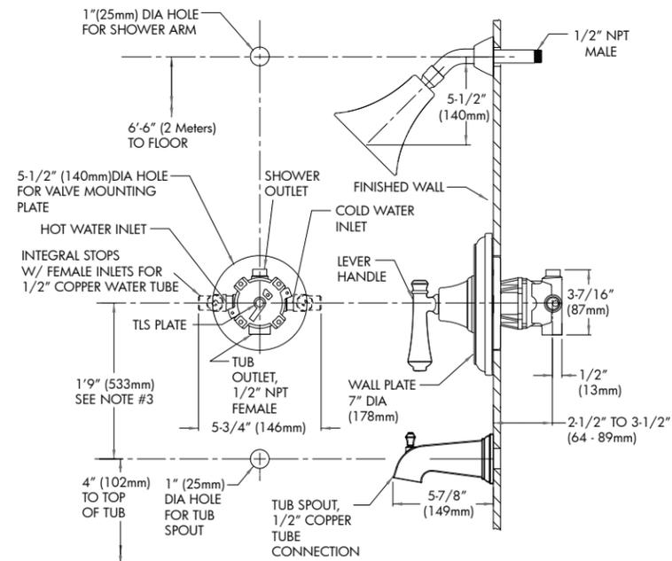
NOTE: 1. All dimensions are in inches (millimeters) unless otherwise specified and are subject to change without notice. 2. Unless otherwise specified, all inlets and outlets are 1/2\"/>
