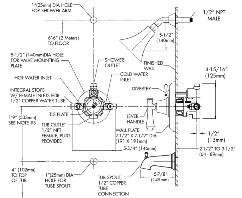
NOTE: 1. All dimensions are in inches (millimeters) unless otherwise specified and are subject to change without notice. 2. Unless otherwise specified, all inlets and outlets are ½" female copper sweat. 3. For ADA mounting locations, consult ADAAG, ANSI A117.1, or static regulations
