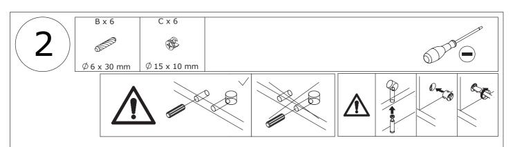
Insert wooden dowel(B) into plate 1, 2 and 3 at first, then attach to plate 4.
