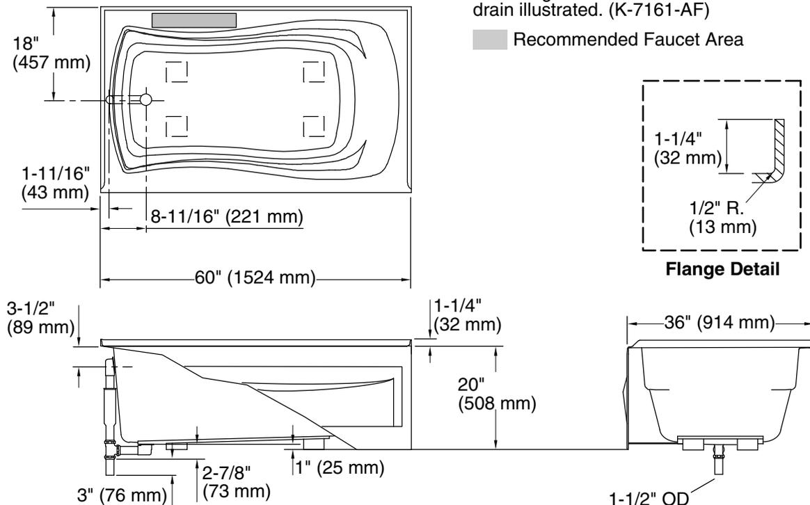
No changes in measurements if connected with drain illustrated. (K-7161-AF)
