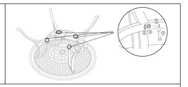
Loosely attach the round support (C) to Table Leg with pre-attached Levellers(B) with washers(②),spring washers(③) and hex nuts (⑤),using the spanner(⑦).
