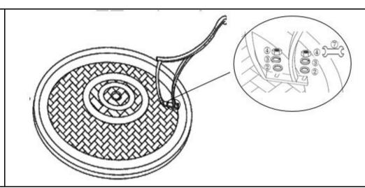
Attach the table leg with pre-attached Levellers(B) to the table top(A) using washers(②),spring washers(③),and nuts(④) with spanner(⑦). **DO NOT OVERTIGHTEN.**
