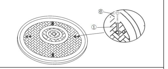
Lay the Table Top(A), facedown, onto a flat, soft, clean surface and lock the mounting positions with bolts(1) by using Screwdriver(6).
