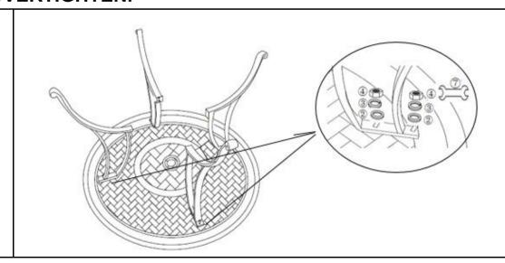
Repeat step 3, attaching the remaining 3 legs to the Table top(A). At this stage, only loosely tighten the Bolts.
