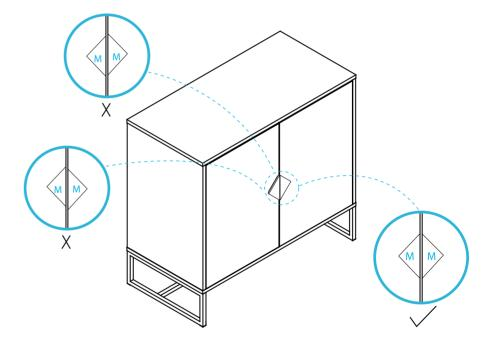
After installation, if the two handles are not aligned, loosen the screws in the back, adjust the two handles to align them, and then tighten the screws back up.
