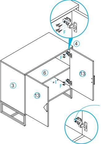
NOTE: If the doors are uneven or there is a gap in the middle, loosen or tighten the screw on the door hinge until they are sitting flush.
