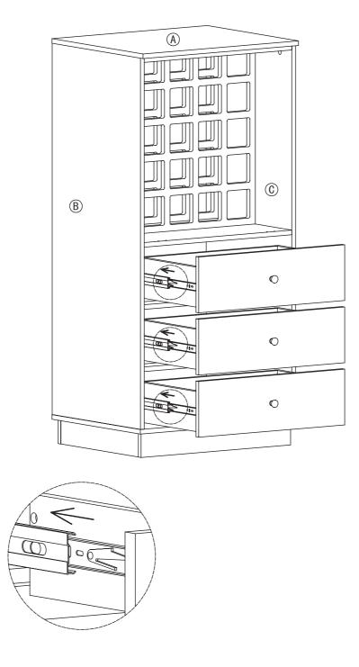
Line up the drawer glides on the drawers on both sides so that they enter evenly into the extended receiving side panel drawer glides as shown then gently push in the drawer until the drawer is secure and slides in and out smoothly.
