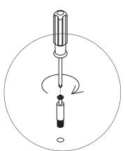
If Cam Lock is too loose, Please adjust Metal Dowel to turn right as drawing.
