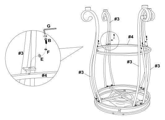
IMPORTANT: DO NOT TIGHTEN COMPLETELY ANY BOLT UNTIL ALL LINED-UP BOLTS ARE CONNECTED TO INSERTED NUTS.
