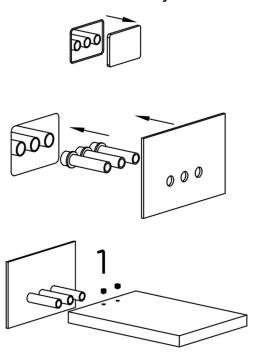
3. After no water leaks fill in the embedded holes and press the panel to the wall. Use the hex spoon to mount the switch handle and the water release handle, and mount the color on.
