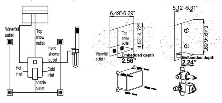
2. Fill in the embedded hole after no water leaks. Screw the water intake on the embedded box after removing the shield and press the panel to the wall. Install the waterfall top spray on the inlet part and lock with a hex key.
