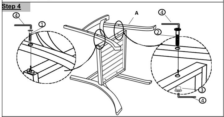
With the help of your partner, turn the Chair over and rest on Right Leg(B). Repeat the same process from the previous step to attach the Left Leg(A). Only loosely tighten the Screws and Bolts.
