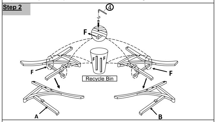
Using Allen Wrench (4) to open 4 Allen screws and 2 Wooden Bars on 2 Leg Panels (A,B) then put them into the trash and continue with step 3.
