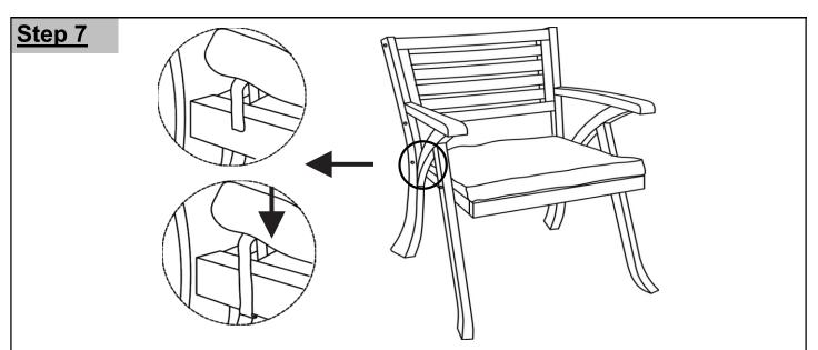
Inspect the Chair and make sure all parts are adequately connected. Place Seat Cushion (E) on to the seat of the Chair using the velcro straps as shown above.
