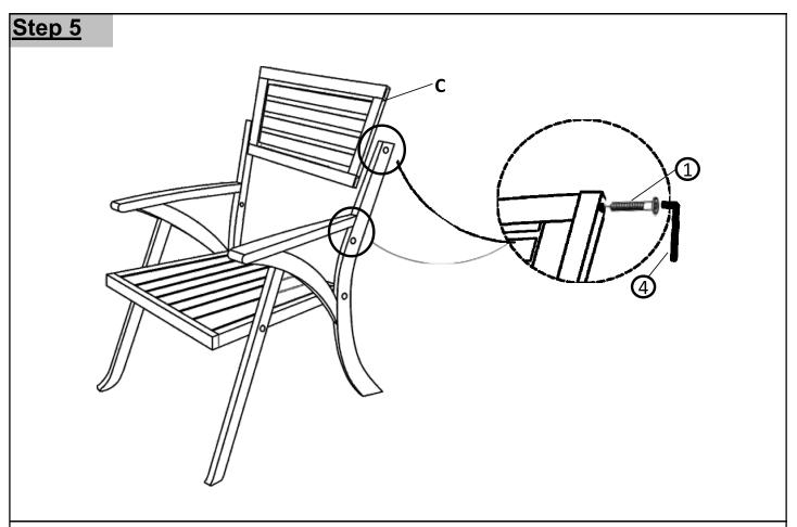
Place Backrest(C) into the housing of Left Leg(A) and Right Leg (B) You may need to apply a little pressure to the Legs, pushing outwards, to enable the Backrest (C) to be slotted into position.
