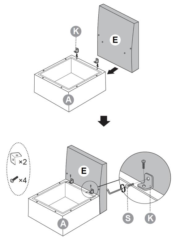
Please tighten the screws to 50% first. Wait for all screws to be fixed and then tighten to 100%.
