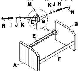
Attached Back Rest(C), Flat Washer(K), Lock Washer(J), Bolt(G) to Left Arm(A) and Right
