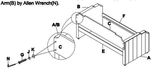
Attached Slats For Daybed(D) to Back and Front Rail (E&F) with Self-Tapping
