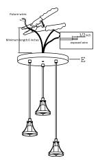
6 » Carefully pass supply wires through mounting plate (C). Secure mounting plate (C) to the outlet box with mounting screws (B).
