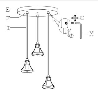
5 » If needed, shorten the extra length of the fixture wires from cords (I) so that they all are at least 6 inches (152.4 mm) long above canopy (E) within the outlet box.
