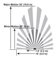
The ASOS32 is designed to replace a standard single pole or multi-way light or fan switch. The sensor uses passive infrared technology to sense human motion in a space and turn the lights or fan ON when occupancy is detected and OFF when the room is vacant. It is ideal for applications in a home where there is a direct line of sight from the sensor to the room.
