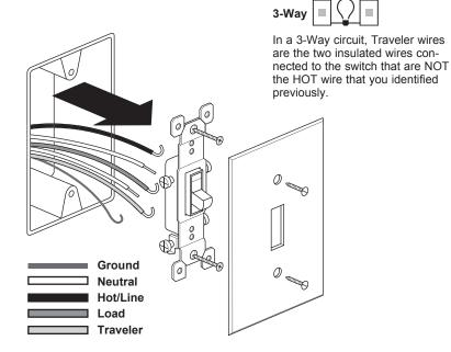
If necessary, cut wires and strip insulation using stripping guide on back of switch.
