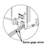
NOTE:When two wires connect to the same terminal on the switch, both wires must be the same gage (12AWG or 14AWG.) If they are not the same gage, you will not have a secure connection
