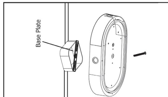
**STEP 4.** Align mounting holes of lamp body to base plate and secure with provided fasteners.
