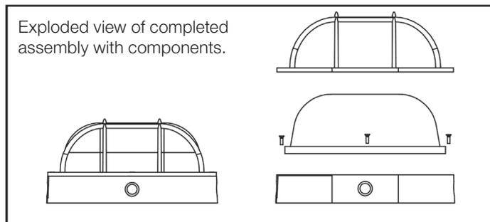
**STEP 1.** Take out led lamp and make sure it is intact. Separate the lamp shade and the base.
