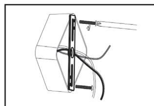
**STEP 2.** Attach the Base Plate to the junction box with the M4 screws.
