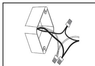
**STEP 3.** Connect the LED fixture to 100–277 VAC 60Hz in accordance to local codes, support fixture while making connections.
