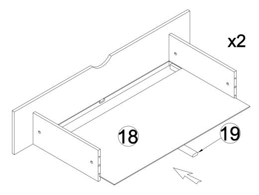
Push detail 19 in first and then push detail 18 into position
