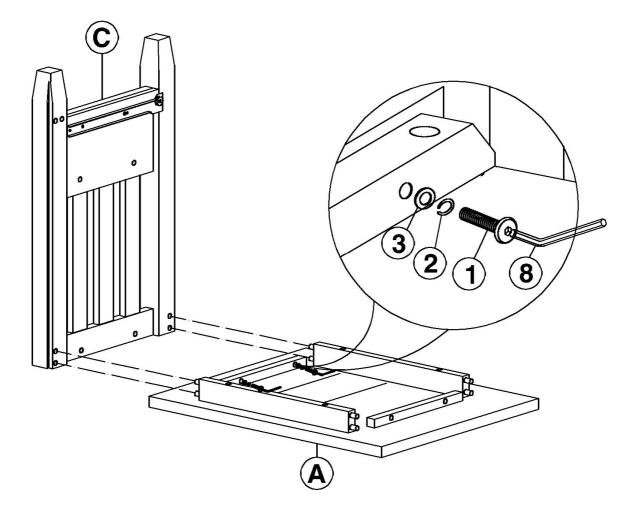
Attach side frames (**C**) to top (**A**) and bottom shelf (**D**) with bolts (1), and washers (2) and (3) as shown below. Tighten with Allen key (8).
