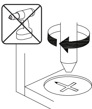
**EN**\_Turn cam lock clockwise to tighten.
