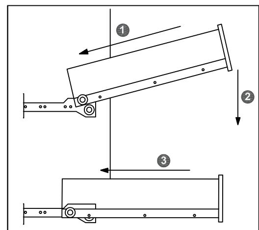
**EN** Be careful to push in the board when the both sides slide way been aligned.
