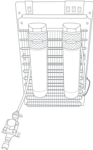
4. Turn on the Valve that was previously shut off. This valve will be located at the connection to the water source or located to the left of the Sediment Filter on the back of the unit.
