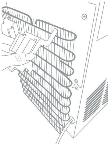
2. Slide the 2 Filter Adapters into each of the Mounting Brackets. Twist the Sediment Filter into the left Filter Adapter and the Carbon Block Filter into the right Filter Adapter. Rotate the filters clockwise to twist them into place.
