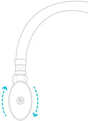
2. Disconnect the current cold water supply line under your sink.
