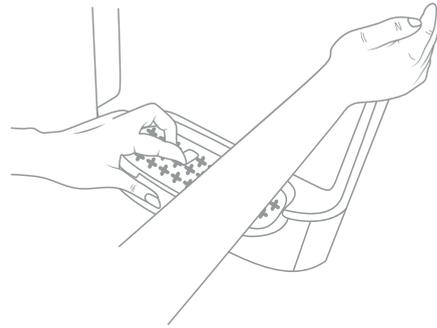
3. Gently pull the drip tray toward you to release it. Once it has been released you can remove the drip tray from the door of the cooler to empty it.
