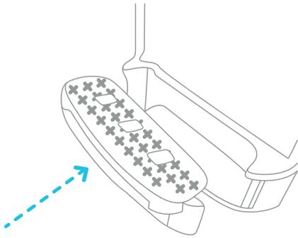
2. To remove the drip tray, place your fingers in the grid of the drip tray with one hand and hold the cooler of the cooler shut with the other.
