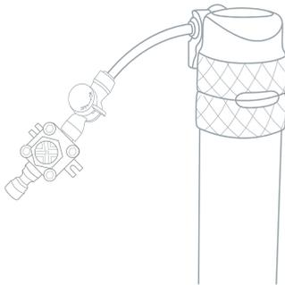
4. Connect the PE Tubing (20'), that is connected to the water source, to the open end of the Valve and Tube Assembly. Make sure that the valve is in the off position (perpendicular to the PE Tubing).
