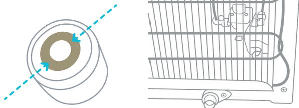
7. Locate the second Small PE Tubing. Connect one end of the Small PE Tubing to the right side inlet of the right Filter Adapter. Connect the other end of that Small PE Tubing to the water inlet (#22).
