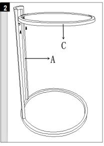
Assemble the Top round shelf (C) to side legs (A) together using 2 screws (E).
