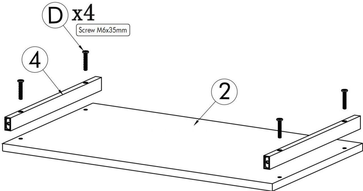
EN-During the assembly, please first half-tighten all the screws into the holes.
