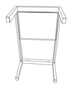
Attach the Table Top Frame(C) to the Right Leg(A) using Bolt(E) and Allen Key(F) as shown in the picture.
