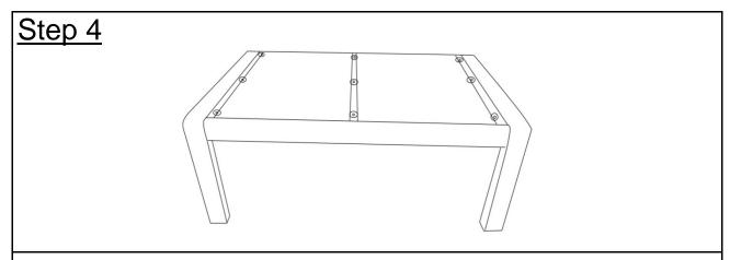
Stand up the table, check stability and then tighten the bolts.
