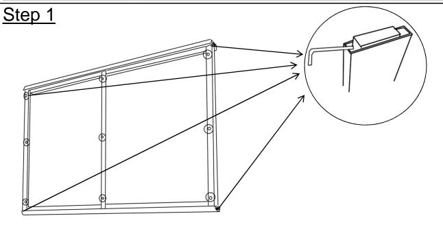
Take out the silders in the four ends of Table Top Frame(C) using Allen Key(F).
