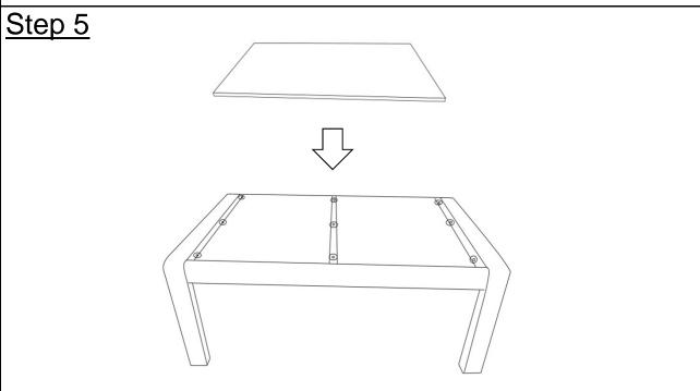
Place the Glass Top(D) on the assembled Table Frame.
