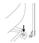
Use socket wrench to loosen the seat rail screw just enough to insert the seat rail mount
