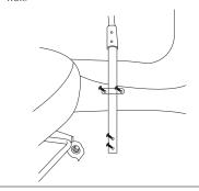
Option 2: screw the floor mount bracket into the vehicles floor/frame and use the fastener bracket to secure the shaft to your vehicles center console wall.
