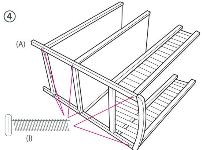
4. Insert the assembled shelves unto one of the End Frames (A). Secure in place using 6 bolts (I). Figure 4
