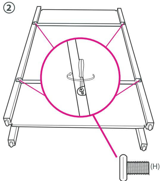
2. Once assembled lay flat with supports facing down and secure shelf insert to both middle supports using four screws. Figure 2.
