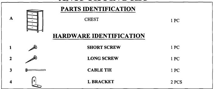
This tip restraint must be attached to a wall stud using long screw enclosed.
